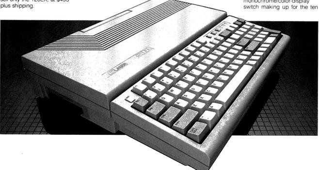
nearly useless function keys. Compared to our first Laser's, the keyboard feels smoother and less plastic—a good improvement, though the sensitive spacebar still puts occasional double spaces between words. The Laser still boots up with Caps Lock on, tricking users into loading their word processors each morning and typing "DEAR SIR"
